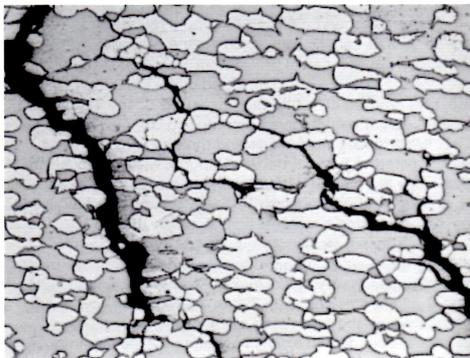
FIGURE 14. Appearance of cracks in superduplex pipe from an alumina plant.
